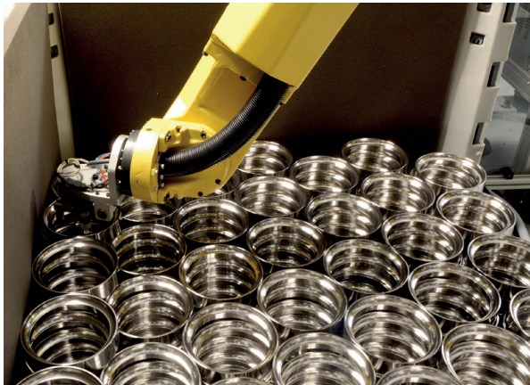
An automated FANUC robot boxes and palletises parts
