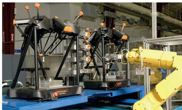
In development - Conroe's new dual Equator automated cell
